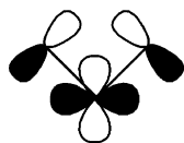
Scheme 4 3c-4e O_t-M-O_t p_\pi-d_\pi-p_\pi bond in cis-MO_2^{2+} unit.
